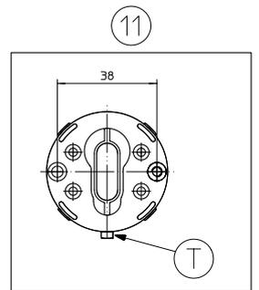
DURING ASSEMBLY, PAY ATTENTION THAT THE HANDLE IS PERPENDICULAR TO THE DOOR STOP.
